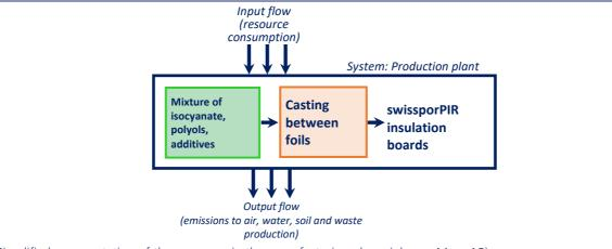
Simplified representation of the processes in the manufacturing phase (phases A1 -> A3)
